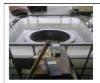
The epoxy is pumped into the water filled form and allowed to cure under replicated conditions
