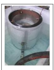
An insulated drum representing the insulated pile splint
