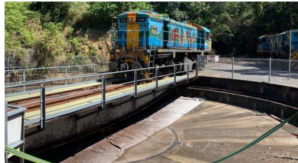
Locomotive moving onto the turntable
