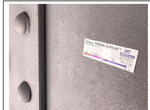
Blast Profile Testing
