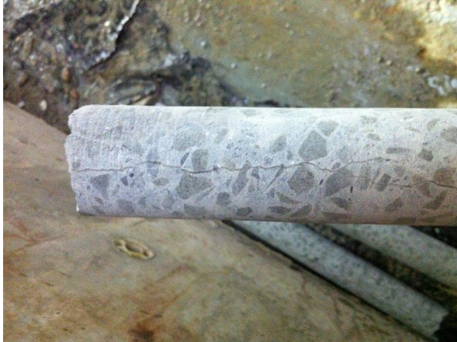
SHOWING DEEP END OF A 1000 MM CORE
